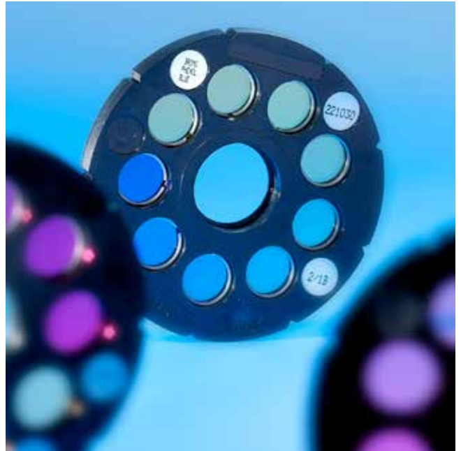
Test disc with colour-stable glass standards
